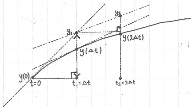
$$y_1 = y(0) + \underbrace{\Delta t y'(t=0)}_{\text{Run} \cdot \text{Slope}} = y(0) + \Delta t f(0, y(0))$$
