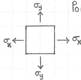
Strain from Stress adds to strain from Poisson's Ratio
