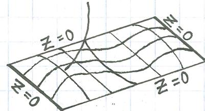
$$z(x,y) = A \sin\left(\frac{mx\pi}{L}\right) \sin\left(\frac{ny\pi}{b}\right) \quad m,n \text{ are } 1,2,3,\dots$$
