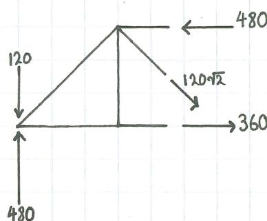
$$\begin{aligned}\sum F_x &= 0 \\ 0 &= F_{FG} + 120 + 360 \\ F_{FG} &= -480 \text{ kN (Compression)}\end{aligned}$$
